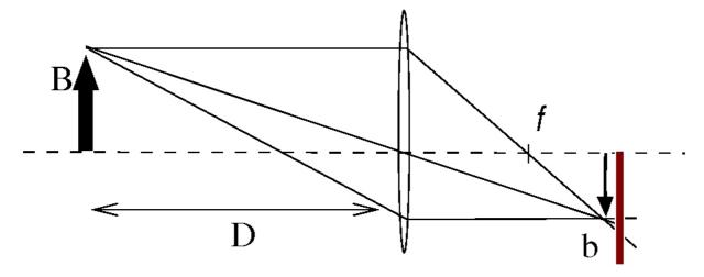
In linear optics light is refracted at the lens in such a way that the Bubble-object 'B' is mapped onto the Bubble-image 'b' at the sensor chip of the camera (red bar). The distance between bubble and lens is 'D'. In Figure 1 of the manuscript the bubbles rise in the volume of observation confined between illumination (1) and box (2). 'f' denotes the focal length and has an impact on the size of the observed volume.
