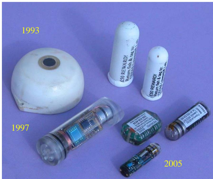
**Fig. 5.** A selection of electronic “archival” or “data storage” tags used to study the movements and behaviour of fish showing the reductions in size over time from Metcalfe et al. (in press, 2009b).
