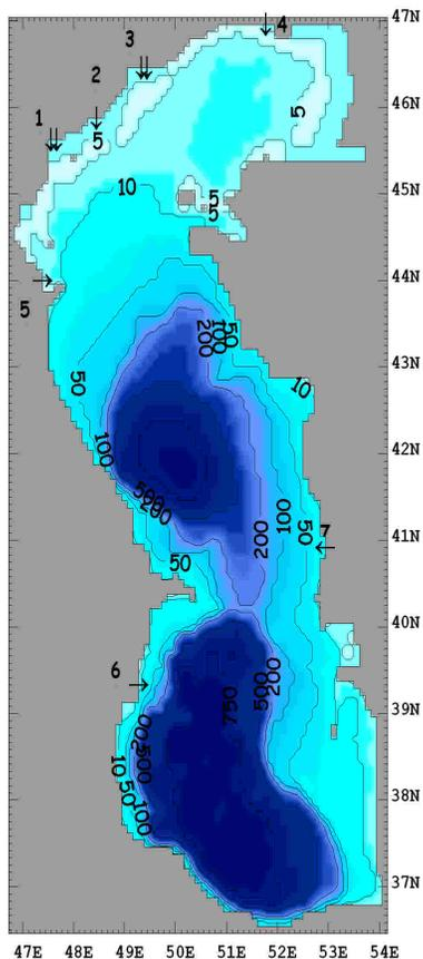
**Fig. 3.** Bottom topography of the Caspian Sea (depths in meters) used in the model. Arrows indicate locations of open lateral boundaries, which include branches of the Volga river: 1 – Bakhtemir (Volga); 2 – Kamyzyak (Volga); 3 – Buzan (Volga), and 4 – Ural; 5 – Terek; 6 – Kura; 7 – outflow to Kara-Bogaz-Gol.
