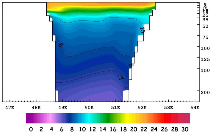
**Fig. 16.** Vertical cross section of sea water density ( $\text{kg m}^{-3}$ ) along  $42^\circ \text{N}$  in July.
