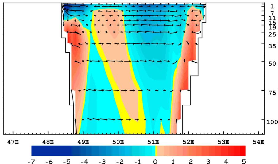
**Fig. 11.** Vertical cross section of currents along 42° N in May: (a) current vectors in the plane of the cross section, (b) isotachs of velocity component perpendicular to the section (northward is positive, southward is negative).
