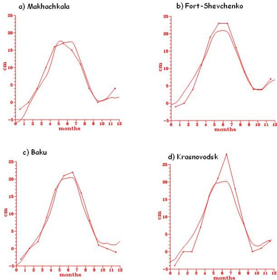
**Fig. 19.** Sea level anomaly (cm) in 1982 at different locations around the Caspian Sea: **(a)** Makhachkala; **(b)** Fort-Shevchenko; **(c)** Baku and **(d)** Krasnovodsk. Smooth curves show model results and the broken lines correspond to observations.
