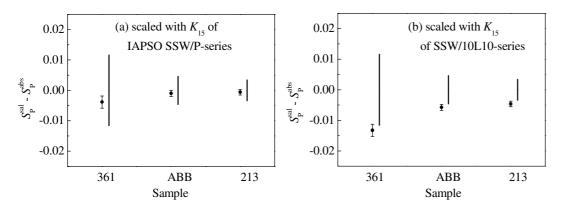
**Fig. 16.** Deviation of Practical Salinity results  $S_P^{sal}$  measured with a salinometer from those calculated from absolute conductivity measurements  $S_P^{abs}$ . Error bars without cross bars are related to zero (deviation) and indicate the expanded uncertainty of  $S_P^{abs}$ , while the error bars with cross bars indicate the expanded uncertainty of  $S_P^{sal}$ . (a) Absolute conductivity results scaled according to Eq. (13) using SSW/P-series, (b) using SSW/10L10 series.
