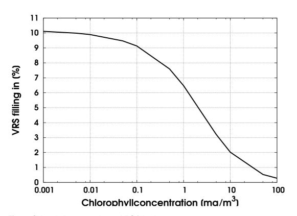
Fig. 3. Chlorophyll concentration vs. VRS filling-in at 397 nm.
