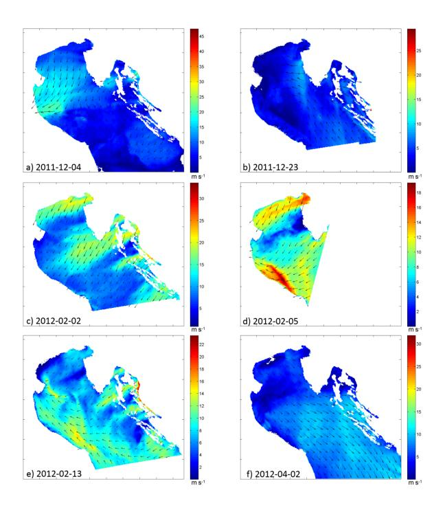
Figure 2. Some of the 15 SAR wind fields available for wave simulation.
