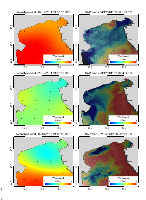
Figure 7. Examples of wind fields with similar patterns between SAR and Reanalysis. SAR winds fields (right) are superimposed to correspondent  $\sigma_0$  SAR intensity.
