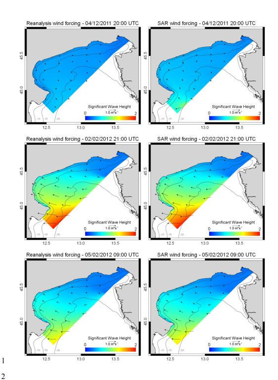
Figure 6. Some cases of waves fields forced with Reanalysis winds (left) and SAR winds (right). Solid isolines are the bathymetric contour lines.
