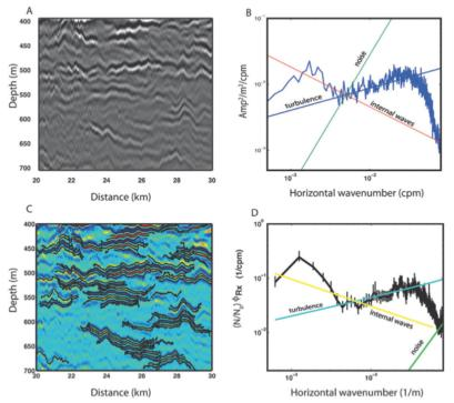
In this figure we see that the slope spectra of the data transform (B) match the slope spectra of the tracked reflectors (D) in general form, namely that horizontal wavenumber ranges reflect internal wave characteristics, turbulent characteristics, and then a drop off where noise does not dominate the data at high wavenumbers. Generally, this shows the information contained in the spectra of the tracked reflectors is also present in the data transform of the seismic data.
