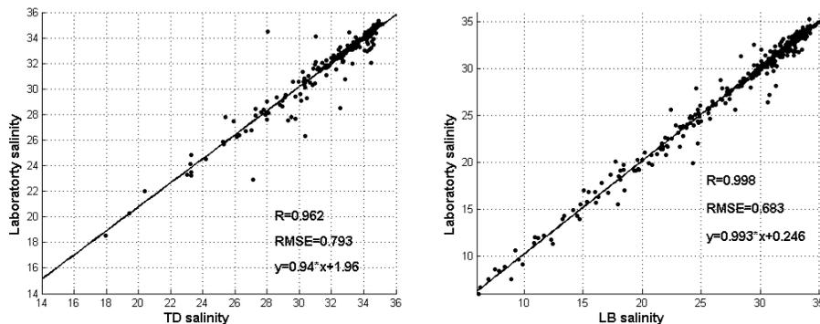
**Figure 3.** Comparison of FerryBox salinity measurements and water sample analyses in the lab for LB (left) and TD (right).
