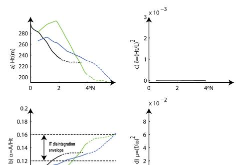
Figure 12. (a) Vertical extension of the waveguide calculated along the waves' propagation paths (see Fig. 9). (b) Nonlinear parameter computed assuming an IT amplitude of 30 m. (c) Nonhydrostatic dispersion for  $L = 100 \, \text{km}$ . (d) Rotational dispersion for the semi-diurnal IT. See text for more details.
