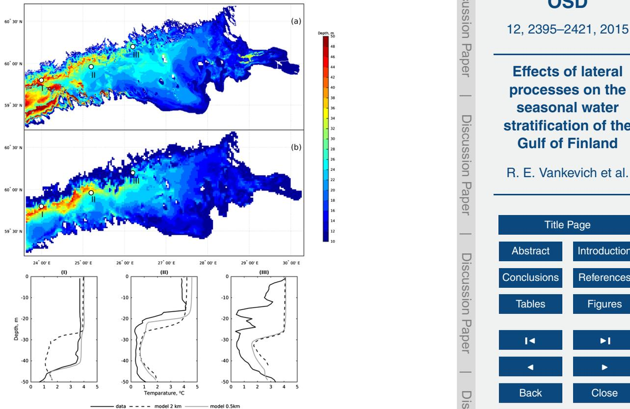
**Figure 5.** Modelled turbocline depth (m) in GOF on 20 May 2011: (a and b) horizontal distributions on grids 0.5 and 2 km correspondently; (i), (ii) and (iii) – vertical profiles of temperature at the locations marked on maps (a and b).
