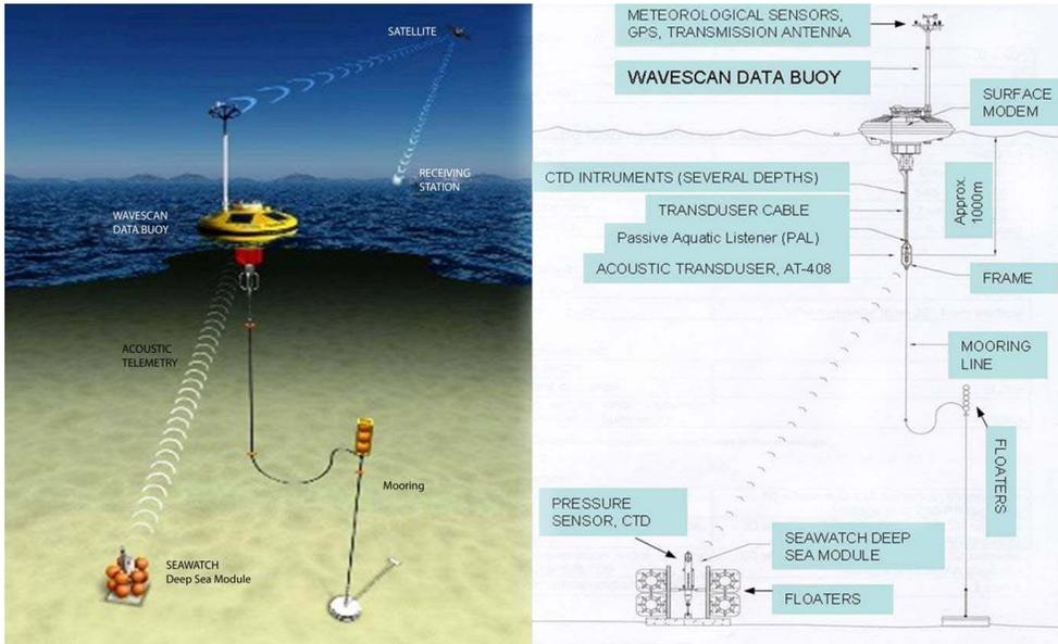
**Fig. 2.** Pylos observatory architecture and components.
