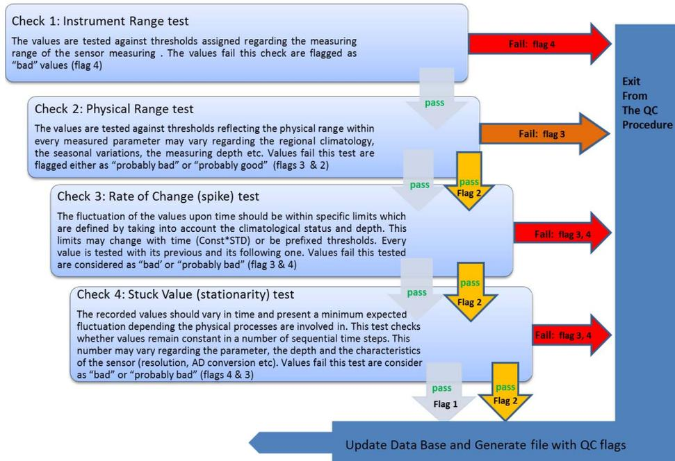
**Fig. 3.** Scheme of real time quality control procedure applied on moored platforms timeseries.
