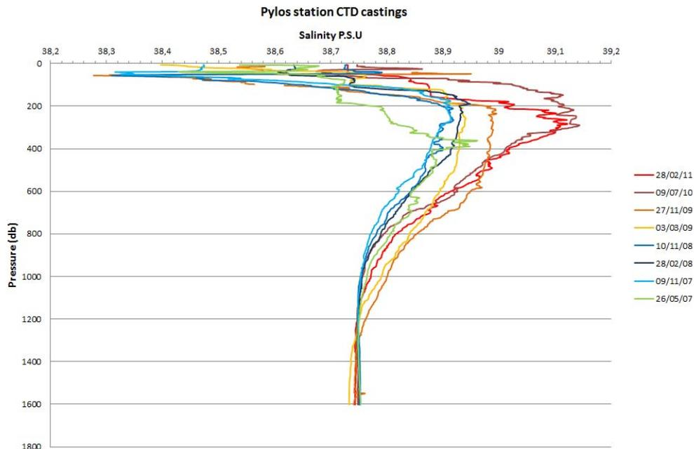
**Fig. 18.** Salinity profiles from 8 different CTD casts during the scheduled maintenance cruises at Pylos station.
