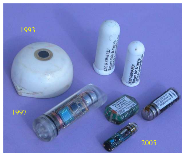
Fig. 5. A selection of electronic “archival” or “data storage” tags used to study the movements and behaviour of fish showing the reductions in size over time from Metcalfe et al. (2009b).
