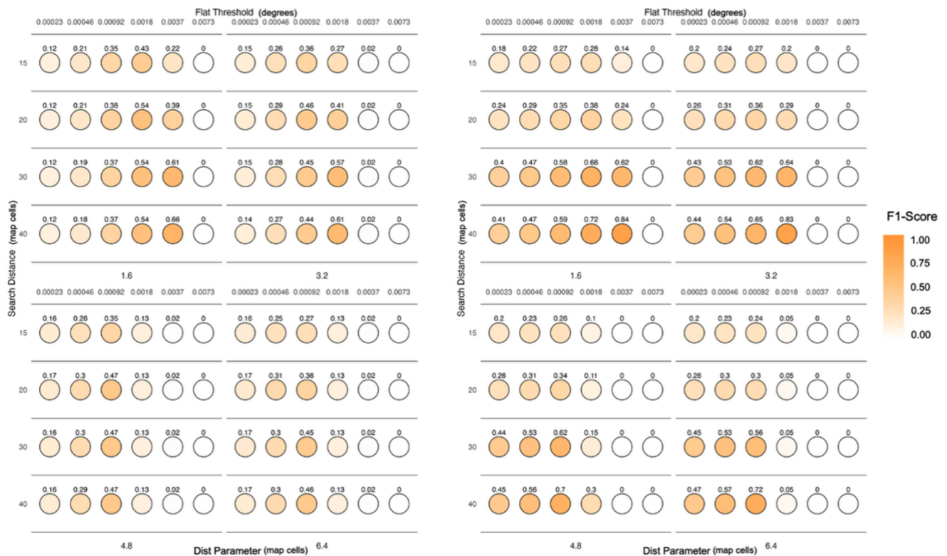
Figure D8. Seasonal performance of all valid geomorphon parameter combinations during austral spring (September–November) for the Weddell Sea (2017), evaluated using daily sea ice concentration fields from the 15th day of each month. Bubble colour indicates the F1-score for months containing one or more reference polynya pixels and the False Positive Rate (FPR) for months in which no reference polynya pixels were present. Bubble size is proportional to the corresponding performance metric. Parameter combinations are arranged according to the search parameter (map cells), flat threshold (degrees), and dist parameter (map cells). The representative parameter tuning case study, 15 October 2017 for the Weddell Sea, is presented separately in Fig. 4.
