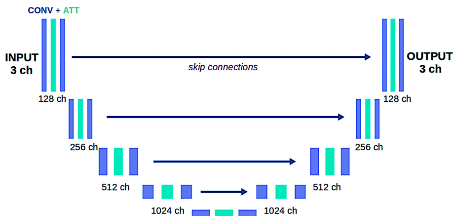
Figure A1. Architecture of the diffusion model, which uses a U-Net with skip connections, attention blocks (in green), and convolution blocks (in blue). The input and generated images are 64 \times 64 in size and have up to three channels for SSS, SST, and SSH depending on the model configuration; the evaluated downscaling target is SSS.
