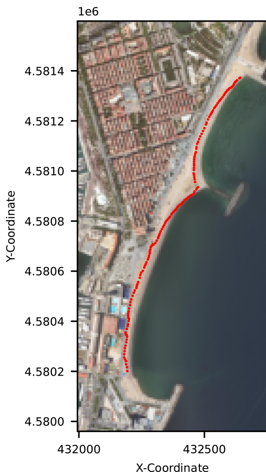
Figure 4. Example of figure received within the e-mail showing the magnitude of flooding – in this case, for a high-intensity event. The red line shows the expected flooding line from the forecast. Orthophoto obtained from the ICGC WMS.
