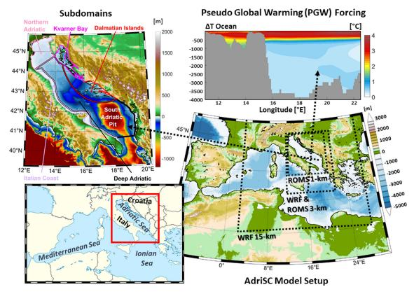
**Figure 1.** Spatial coverage and horizontal resolution of the different grids used in the AdriSC climate model setup including the topobathymetry of the AdriSC 1 km model with the locations of the five subdomains (coloured polygons) used in this study and the pseudo-global-warming temperature ocean forcing imposed in the AdriSC 3 km model southern boundary for the extreme warming simulation.
