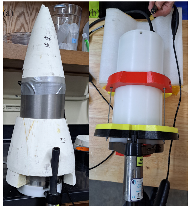
Figure 2. SG HydroC CO 2 sensor mounting designs. (a) Titanium SG HydroC CO 2 (rated to 1000 m) in a custom syntactic foam coat and (b) polyoxymethylene SG HydroC CO 2 (rated to 300 m) with brackets.
