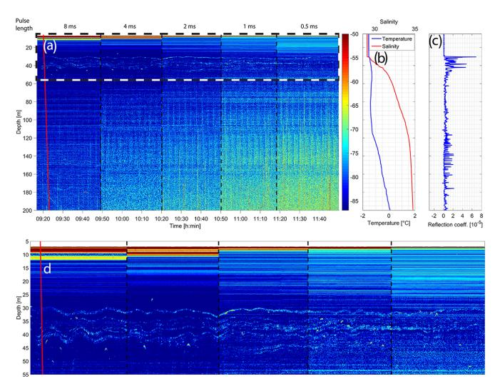
**Figure 4.** Comparison of EK80 data with different pulse lengths. Data were acquired on 26 August 2016 at 140.6° W, 86.8° N. (a) EK80 echogram. (b) CTD profiles showing temperature (blue) and salinity (red). (c) Reflection coefficients derived from CTD data. (d) Enlargement of dashed box in (a). In (a) and (d), the vertical red line is the CTD position and the vertical dashed black lines indicate changes in pulse length (decreasing from 8 to 0.5 ms).
