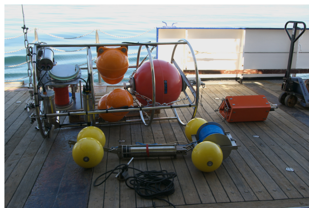
Figure 6. Mooring components laid out on deck before the second deployment in July 2010. Recovery system with acoustic releaser (front), underwater winch (back left) and profiling platform with instruments (back right).
