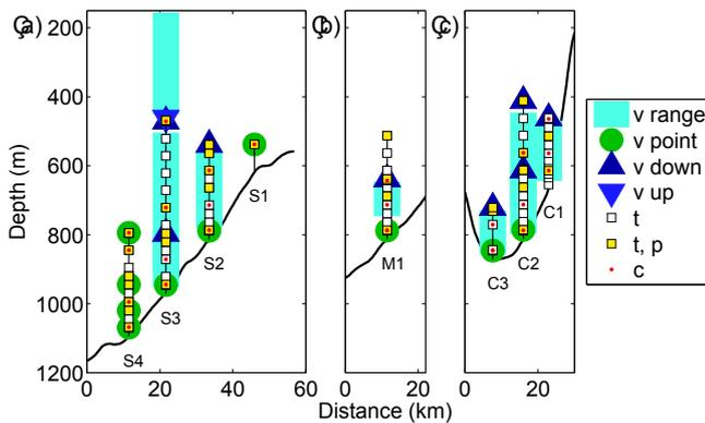
**Figure 2.** Mooring arrays: (a) section S, (b) mooring M1, and (c) section C. Each section is viewed looking downstream (southernmost mooring on the left). Sensors for temperature, pressure, conductivity, point velocity, as well as the range covered by the upward- and downward-oriented acoustic velocity profilers, are indicated.
