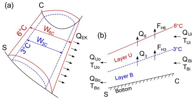
**Figure 15.** A schematic view of the overflow plume between sections C and S, demonstrating the components of the heat budget. The 3°C isotherm marks the upper limit of the bottom (B) layer, and the 6°C isotherm the upper limit of the upper (U) layer.
